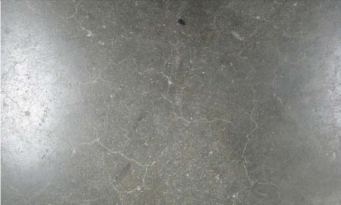
Photo 1: Showing crazing on control slab #1 subjected to 200° F with rapid air movement above slab.
