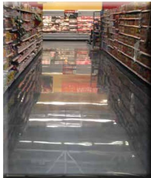
SmartFloor™ is only usable with Ameripolish SR2 due to its fully penetrating nature. SmartFloor™ Pads are composite resin abrasives that clean and hone the surface on a daily basis to provide the floor with its highest possible DOI even after the installer has left.
